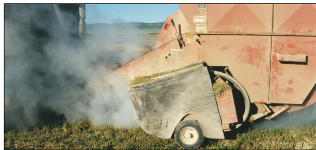
Figure 2. Steam re-hydration of alfalfa at baler pick-up.
