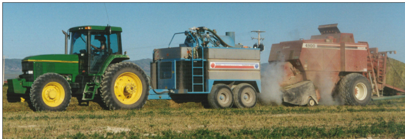
Figure 1. Steam generation unit located between the tractor and large square baler with steam applied at baler pick-up (Staheli West, 2013).
